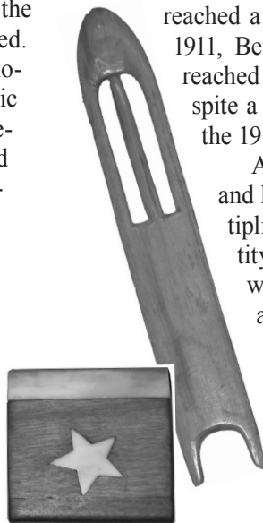
Wooden mesh stick with bone inlays, left, and wood mesh stick were used for weaving, repairing and measuring the size of the gill net pockets and joined areas. The tools, carved by Charles Berg in about 1925, are now owned by his step-granddaughter Carol Steele, of Gresham, Oregon.
